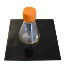
Adhesive mat, black. Strong adhesive special mat for easy attachment of different vessels onto the shaking platform or tray. Max. shaking speed: up to  $250 \, \text{min}^{-1}$  (depending on shape and weight of the vessel as well as on the shaking amplitude). Dimensions:  $200 \times 200 \, \text{mm}$ , the mat can be cut or trimmed with scissors.
