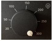
Turn the left-hand control knob clockwise to increase the shaking frequency and anti-clockwise to decrease the shaking frequency.
