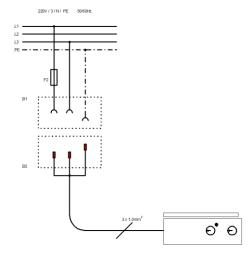
Varioshake Shaking Apparatus in 230 V with mains supply 230 V / 3  $\sim$  / PE / 50 / 60 Hz connected through 3-pole shock-proof plug system.
